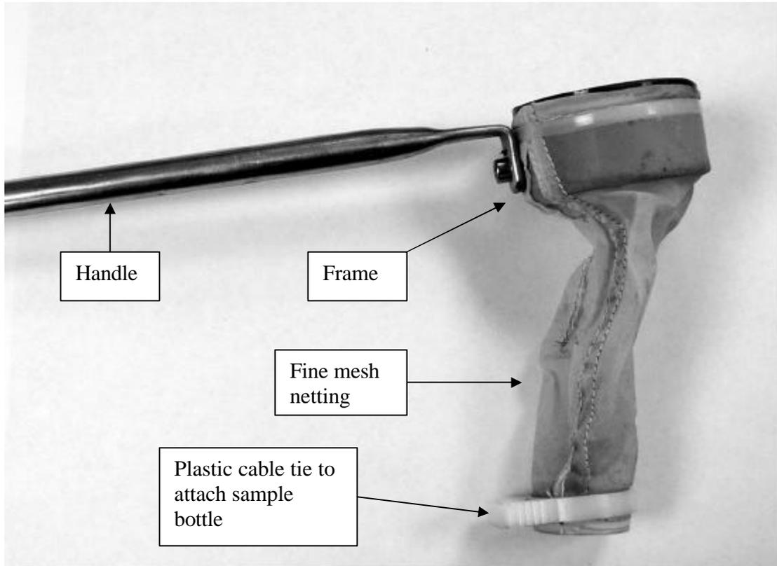
**Fig. 2.2. Photograph of sampler for vertical hard surfaces.**
